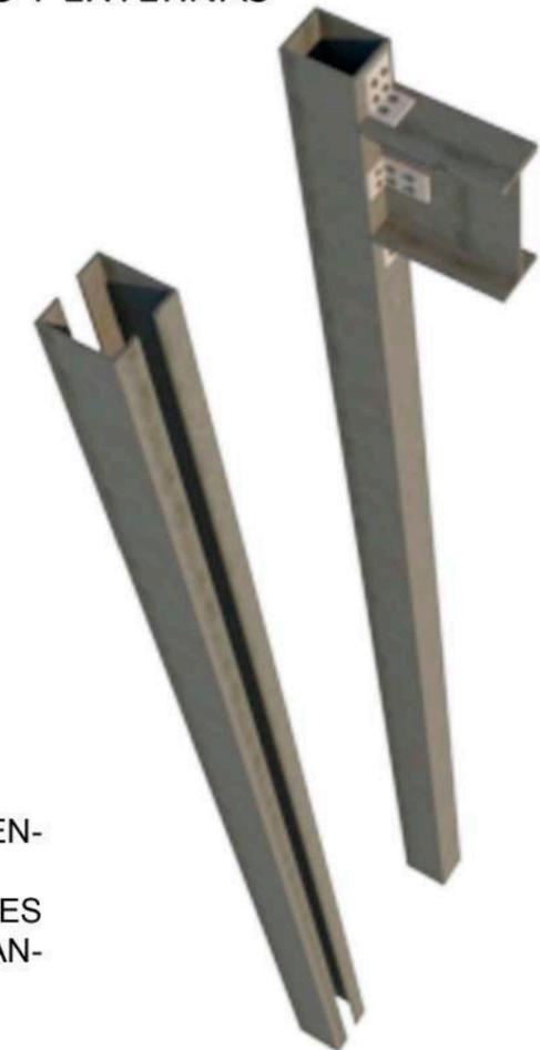
LAS COLUMNAS DE ACERO SE FORMAN UNIENDO DOS PERFILES C.
