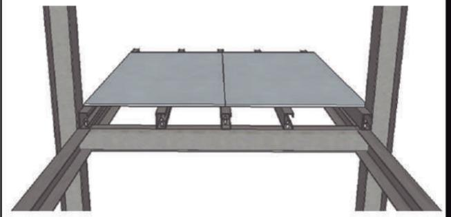
UNION ENTRE COLUMNAS ,VIGAS PERFIL H Y ANCLAJE
