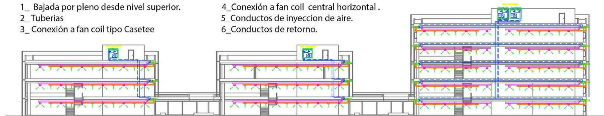
DETALLE FAN COIL CONDENSADO POR AIRE
